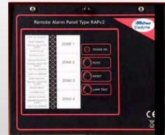
When in an alarm state, the unit will sound the alarm and flash the corresponding indicator on the front panel in order to alert the operator. Depressing the 'MUTE' button will silence the alarm and active channel indicators will cease to flash, holding steady in the 'ON' state. Pressing 'RESET' button will return all inactive fault channels to the 'STANDBY' state, clearing the corresponding indicators.
